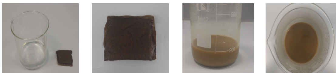
Figure 3. Complete solubilization of the film with carob powder into composition (A4R) after 30 " maintenance in hot water (80 °C)
