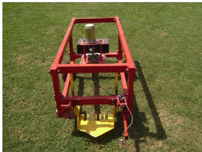
Fig. 1. Head of onion harvester including control depth system.
