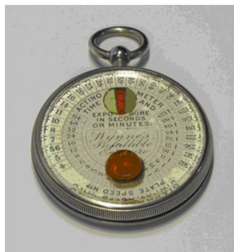
Fig. 9. Actinometer from 1903 [6].
