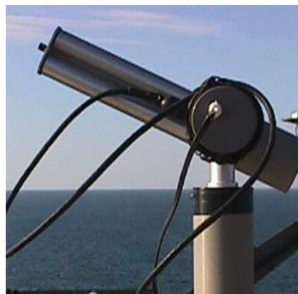
Fig. 16. AERONET Photometer [5].
