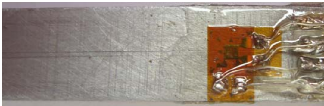
Fig. 5. Strain gauge in T-shape apply on the plain sample.
