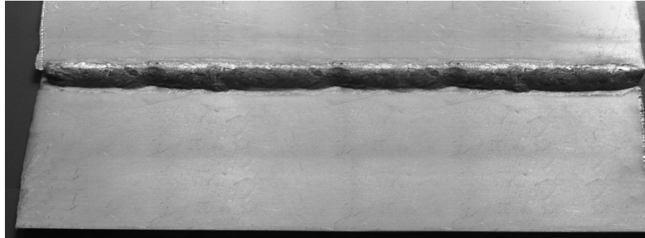
Fig. 1. Fe–Cu–Al brazing joint.
