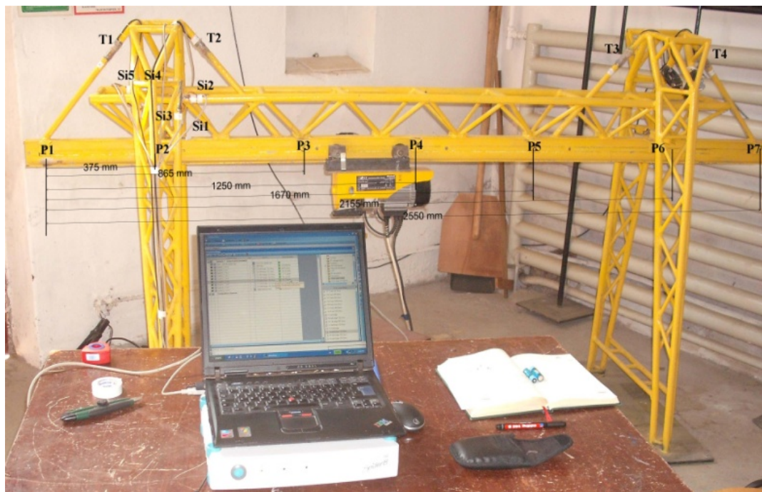
Fig. 1. The assembling scheme for the measurement of forces in windbracings and of stresses in the fracture sensitive elements [1].
