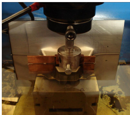
Fig. 3. Cutting samples by EDM.
