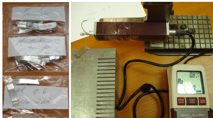
Fig. 4. Prepared samples and Mitutoyo SJ-20 roughness device.
