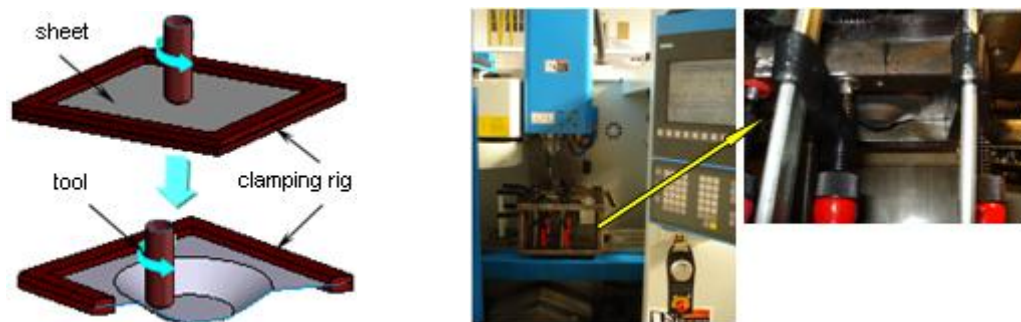
Fig. 1. Principle of the single point incremental forming process.
