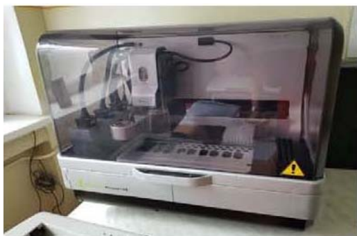
Fig. 1. The Adaltis Personal Lab automatic analyzer for the determination of antigen HBs and anti-HCV antibody
