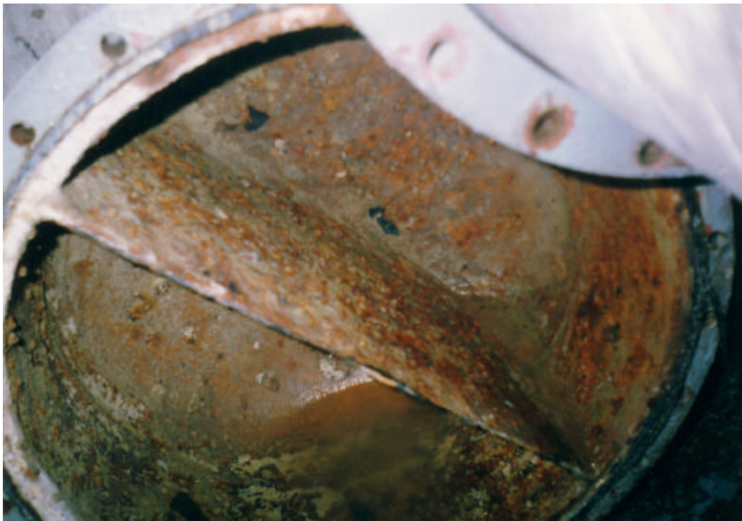
Fig. 11. Ammonia carbamate solution cooler: water turning end after washing
