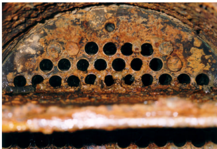
Fig. 7. Water inlet tube sheet of the C 3 - C 4 fraction cooler
