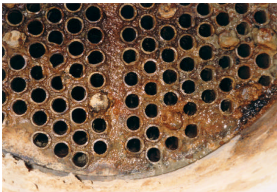
Fig. 6. Water inlet tube sheet of the C 4 fraction cooler
