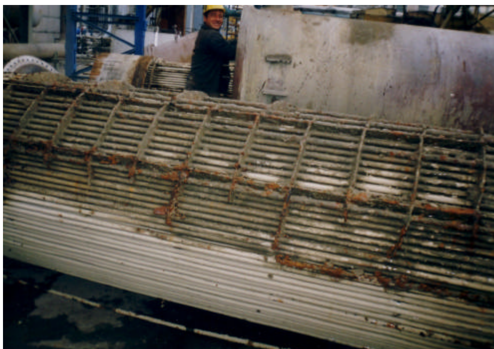
Fig. 14. Tube bundle of a wet CO 2 cooler right after dismantling
