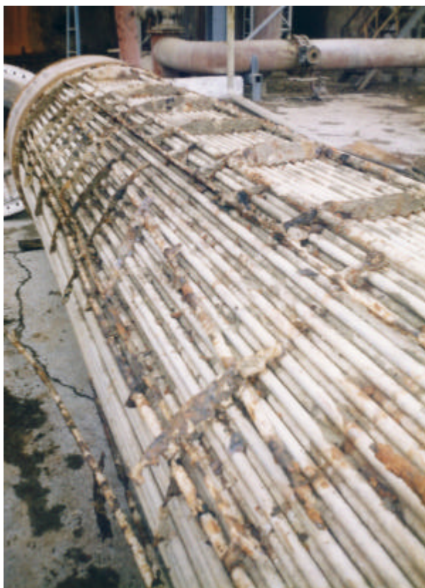
Fig. 15. Severe galvanic attack of mild steel baffles and rods in contact with the 316 SS tube bundle
