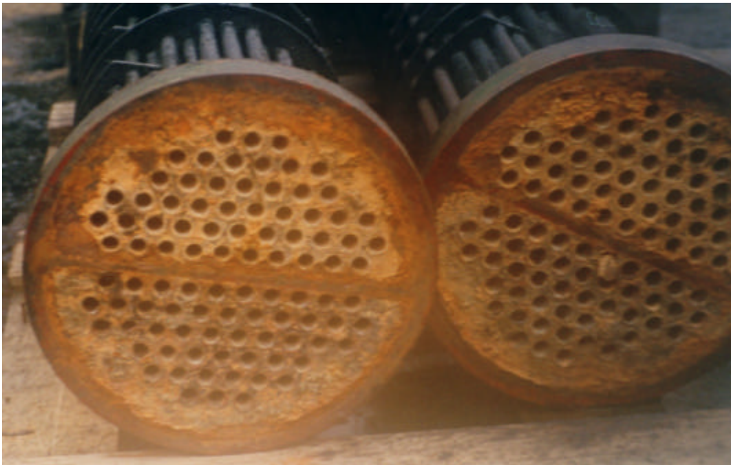
Figure 17. Tube sheets of the oil coolers equipped with copper tubes
