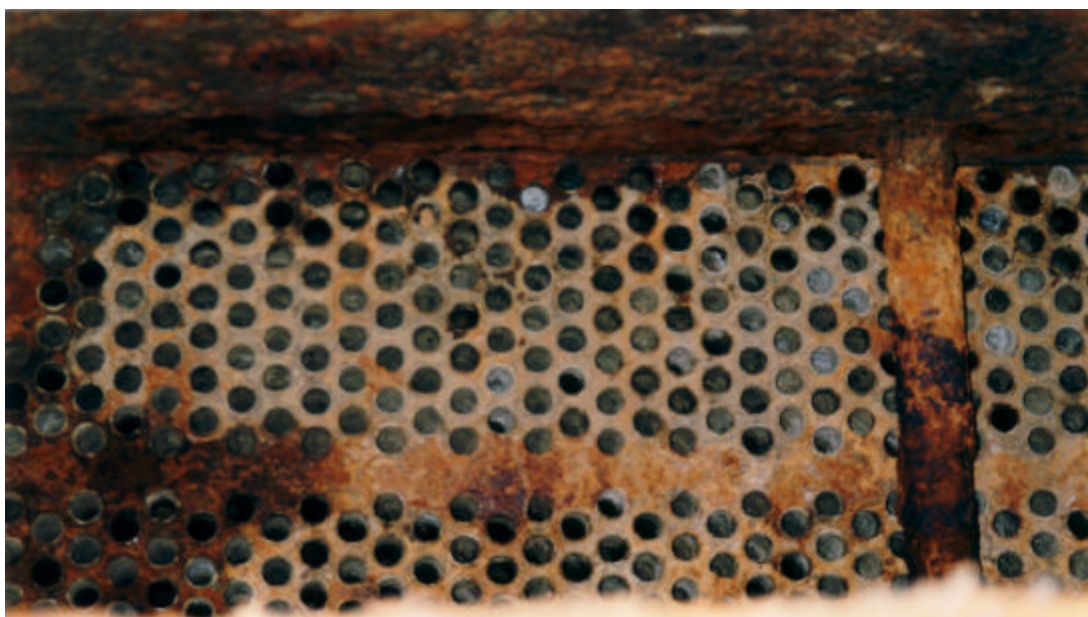
Fig. 3. Galvanic attack at the inlet water box of the fraction C 3 cooler
