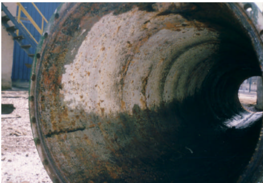
Fig. 16. Mild galvanic attack of the carbon steel shell of a CO 2 cooler (urea plant), due to the contact with 304 SS baffles
