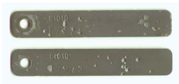
Fig. 5. Corrosion due to the SRB on carbon steel
