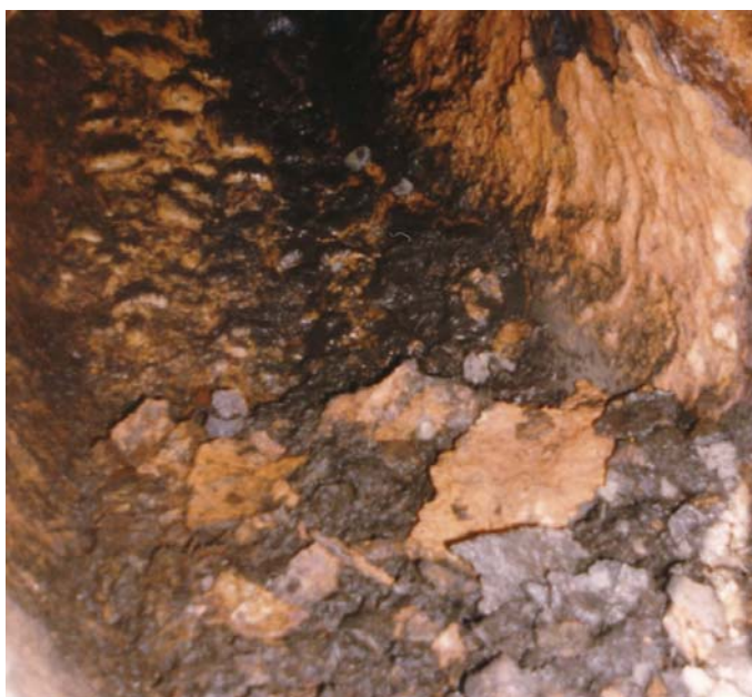
Fig. 7. Tubercles in a recirculated water pipe (System no. 3)
