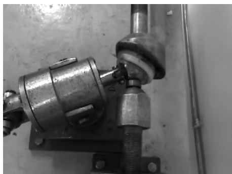
Figure 5. Installation for testing the tribological parameters
