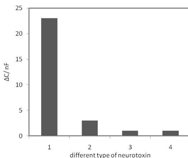
**Figure 7.** Comparison of BoNT/A (1) response with rBont/B (2), Bont/AHC (3) and rBont/E (4) in concentration of  $0.1 \text{ ng}\cdot\text{mL}^{-1}$  on aptamer/RGR modified Cp electrodes in  $0.1 \text{ M PBS}$  solution ( $\text{pH} = 7$ ) by capacitance method
