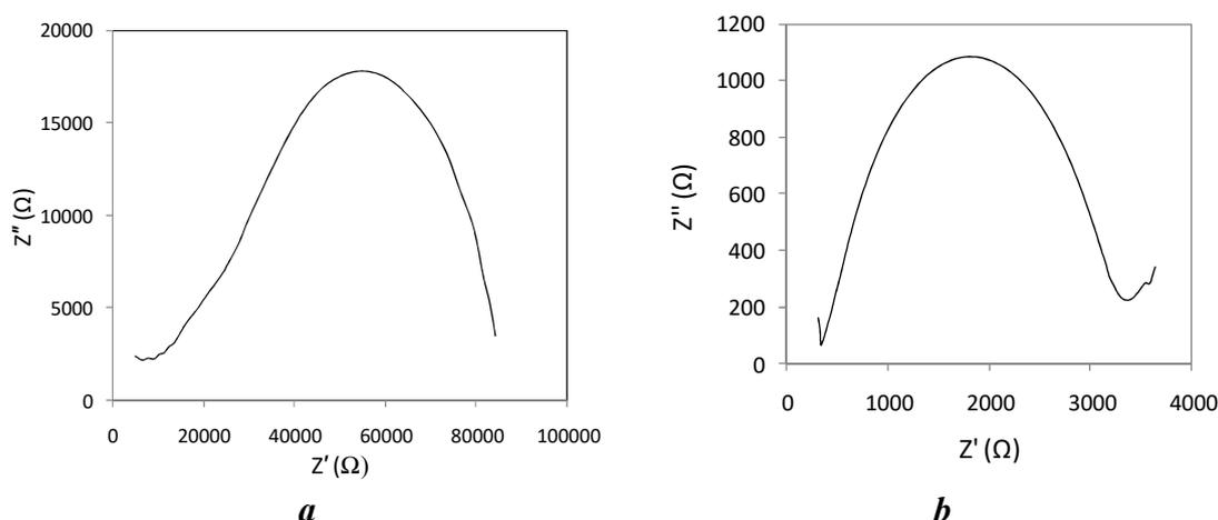
**Figure 5.** EIS of  $1.0 \text{ mmol}\cdot\text{mL}^{-1}$  hexacyanoferrate (II) / (III) (1:1 mixture) on Cp electrode (a) and RGr + Cp electrode (b) in  $0.1 \text{ mol}\cdot\text{mL}^{-1}$   $\text{KNO}_3$  and  $0.1 \text{ mol}\cdot\text{mL}^{-1}$  PBS solution ( $\text{pH} = 7.4$ )
