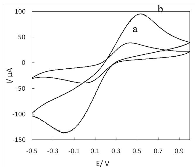
**Figure 4.** CVs of  $1.0 \text{ mmol} \cdot \text{mL}^{-1}$  hexacyanoferrate (II) / (III) (1:1 mixture) on Cp electrode (a) and RGr + Cp electrode (b) in  $0.1 \text{ mol} \cdot \text{mL}^{-1} \text{KNO}_3$  and  $0.1 \text{ mol} \cdot \text{mL}^{-1} \text{PBS}$  solution ( $\text{pH} = 7.4$ ) (the scan rate is  $100 \text{ mV} \cdot \text{s}^{-1}$  at air saturated condition)
