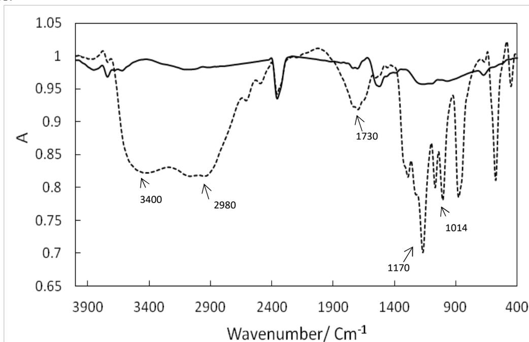
*Figure 3. FTIR spectra of graphene oxide (---) graphene (—)*
