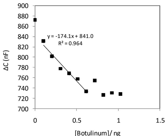
**Figure 6.** Calibration curve of BoNT/A determination on aptamer/RGR modified Cp electrodes in  $0.1 \text{ M}$  PBS solution ( $\text{pH} = 7$ ) by capacitance method
