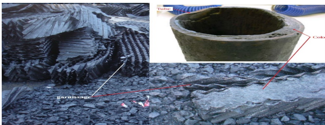
Figure 2. Filling of coke in a tube of oven and bed of trim
