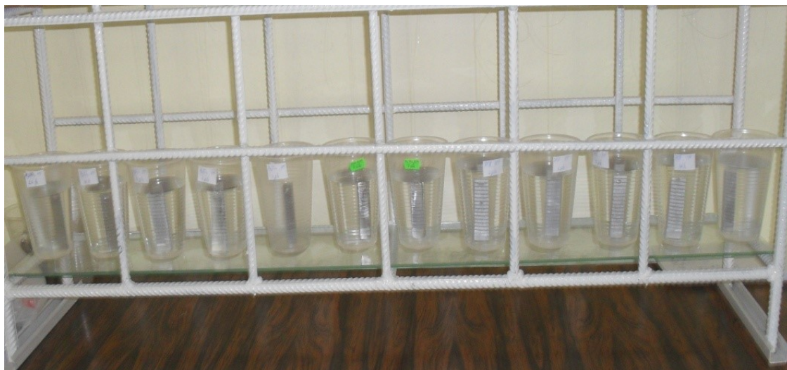
Figure 1. Experimental assembly for corrosion determination
