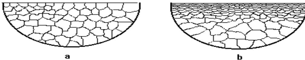
Fig. 1. Crystalline structure of the superficial layer in the case of steel: a – boring sample; b – rolled sample [1].
