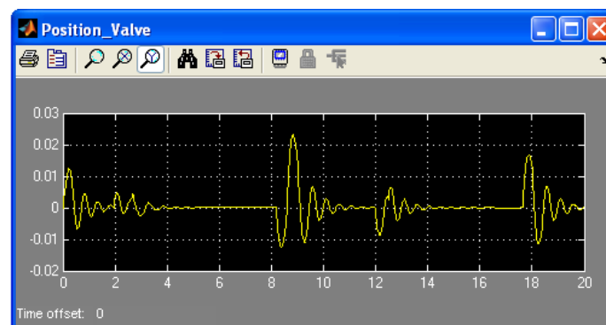
Fig. 8. Position of servovalve.
