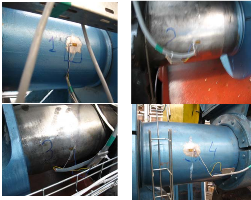
Fig. 4. The four measuring points on the columns.
