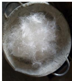
Fig. 1. 54mm synthetic macro fibre (Polypropylene).
