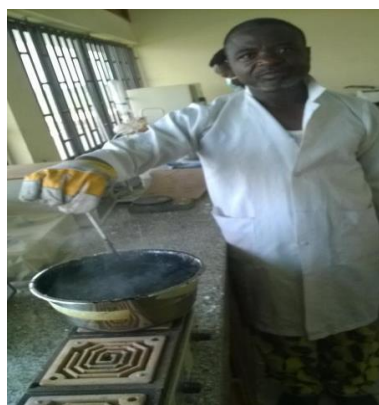
Fig. 1. Melting of ground EPS in bitumen.
