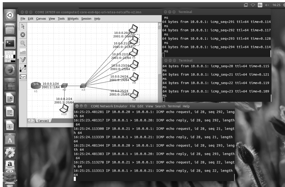
Fig.2. Running the experiment: Two workstations, simultaneously exchanging ICMPs with the router are monitored by the n10 station
