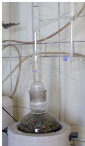
Photo 1. Clevenger apparatus (source: http://homepages.ihug.com.au/~panopus/lab/labequip.htm )
