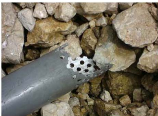
Fig. 2a. The destroyed survey tube
