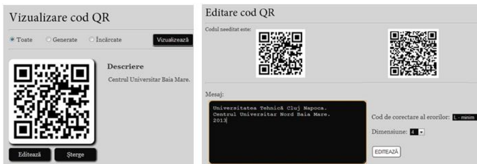
FIG.4. In the left side is the window where the user has the possibility to visualize all its personal QR codes by default or just the generated or the uploaded ones. In the right side is the editing window where the user could modify an existing code using another text and/or another error code and/or another dimension of the future code; both QR codes , initial and its modified version are also illustrated.
