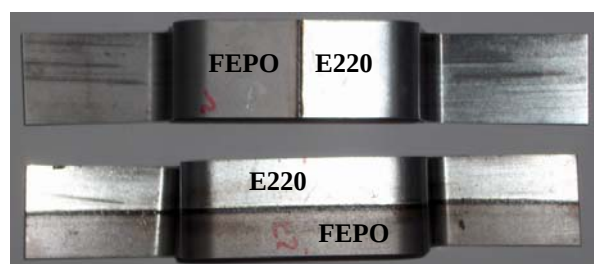
Fig. 6. Parts made by TWBs with transversal and longitudinal weld line
