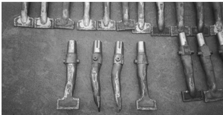
Fig. 3 The classic tamping tools type P & T 09 – 32 CSM – curved plated (armed) on the active part by manual and electrically welding with two types of metallic covered electrodes, which were recommended by the producers for the high abrasive and shock resistance
