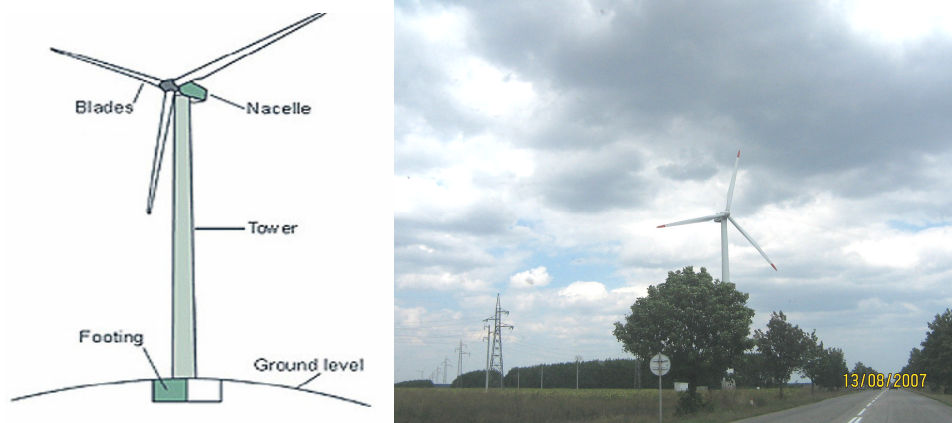
Fig.2. A simplified schema of a wind turbine
