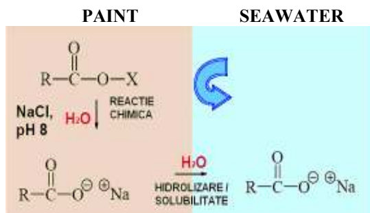
Fig. 1: The general mechanism of auto-polishing process
