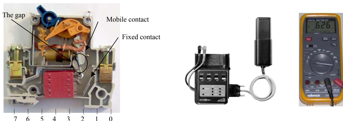
Fig. 1: The components of experimental stand: automatic circuit breaker, Metra Hit FMA1, DVM345di multimeter.
