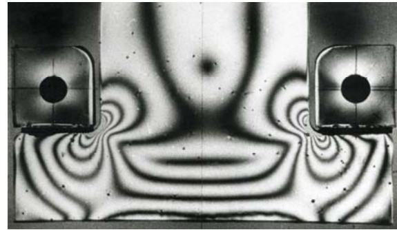
Fig. 2 The isochromatic fringes for R_2 = 3 mm
