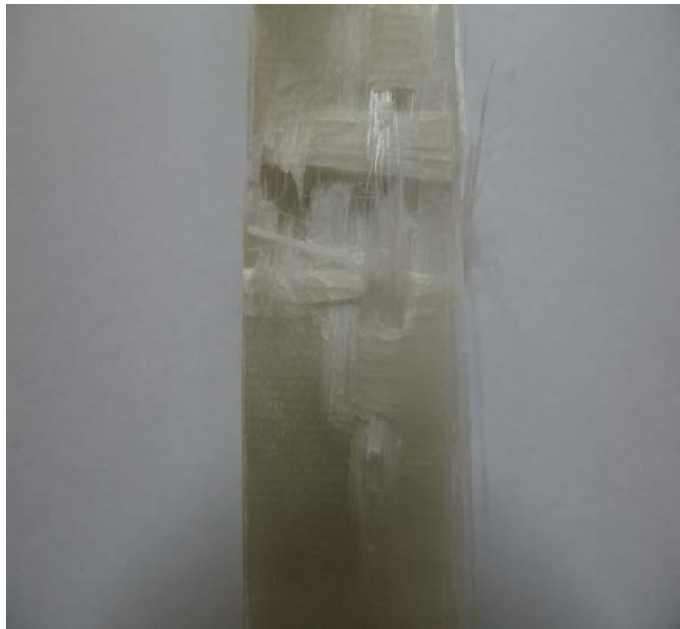
Fig. 2. Front view 1 of the failure mode
