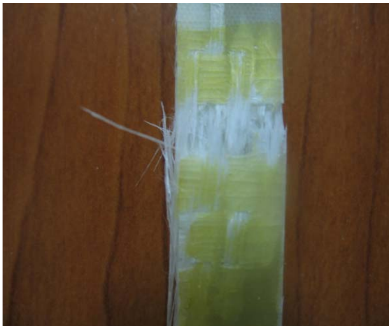
Fig. 3. Front view 2 of the failure mode
