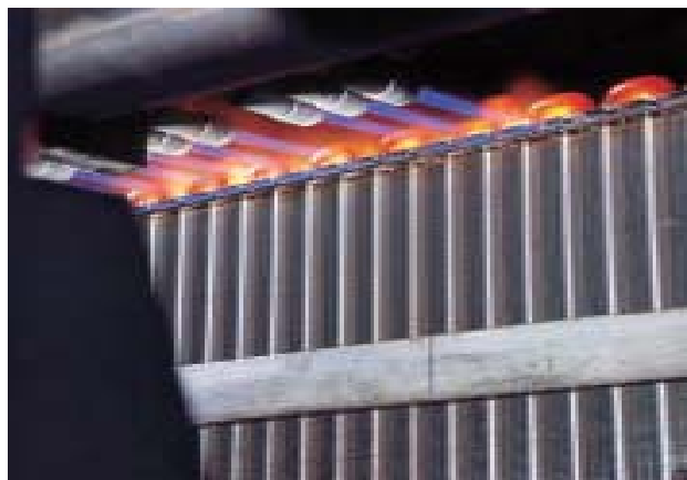
Fig. 1 Automated torch brazing system
