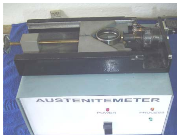
Fig. 2. The general view of the austenite-meter
