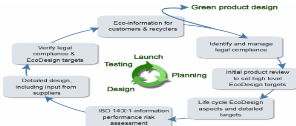
Fig. 1 Flow chart of green product design and eco-design steps, ISO 14001 appliance.
