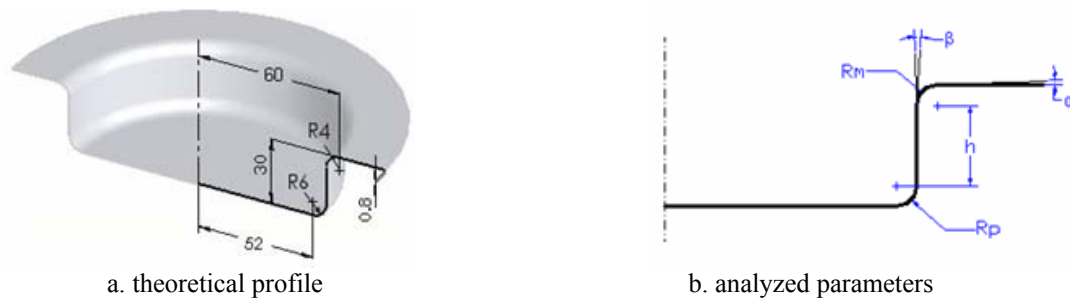
Fig. 2 Geometry of the cylindrical parts
