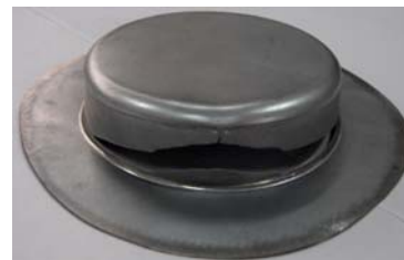
b. material fracture
