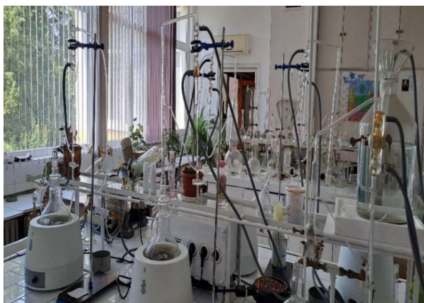
Figure 3. Laboratory glass apparatus for hydrodistillation of the British Pharmacopoeia, modified by Balinova and Dyakov [22] (authors' images)
