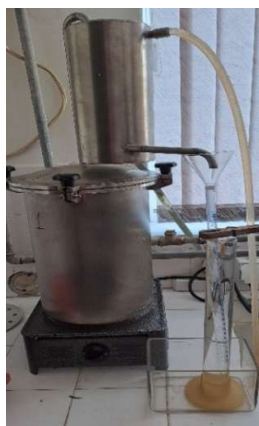
Figure 2. Laboratory apparatus for steam distillation (authors' images)
