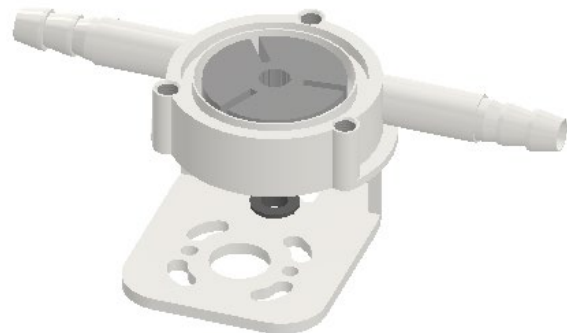
Fig. 7. The assembly between the base and rotor.
