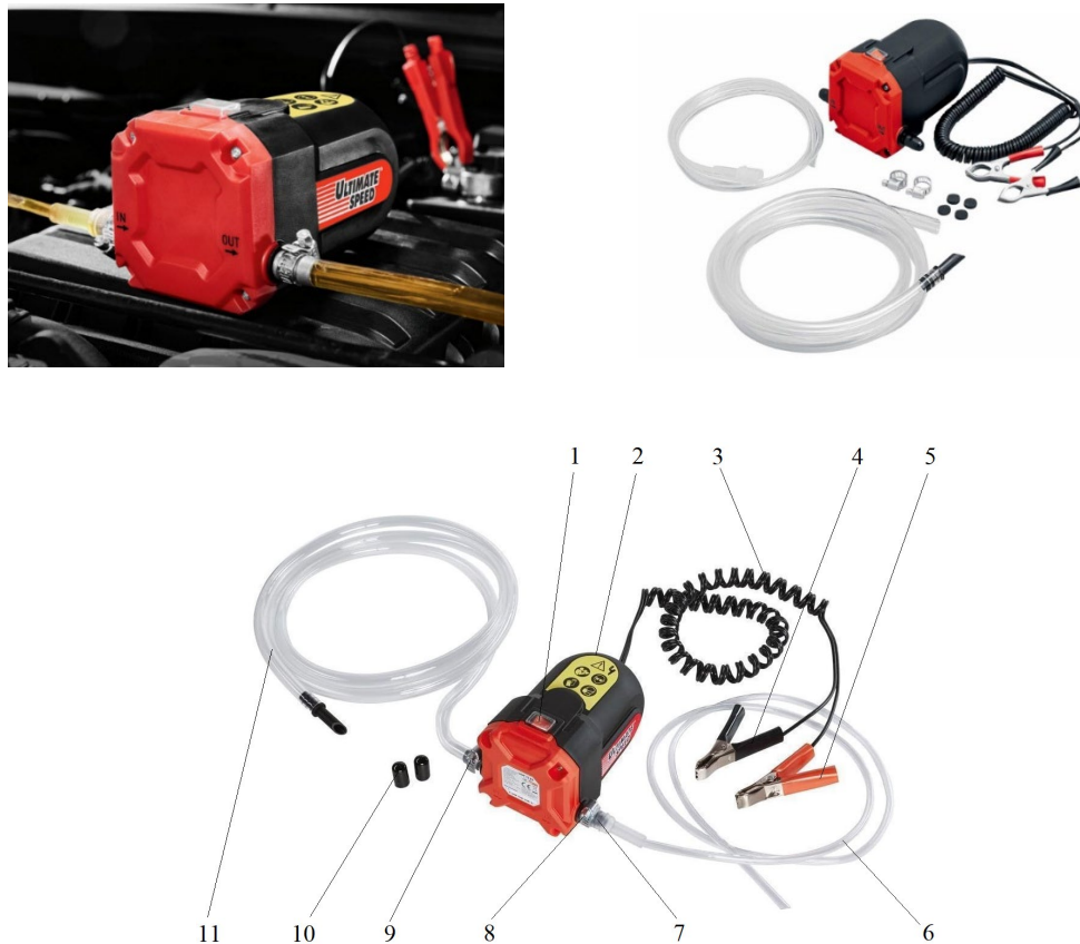
Fig. 2. UOP 12 C1 oil pump [13]: 1 - on / off switch; 2 - pump housing; 3 - battery connection cable; 4 - negative terminal (-) (black); 5 - positive terminal (+) (red); 6 - suction hose, diameter 6 mm; 7 - connector for the discharge hose ( OUT ); 8 - hose clamp; 9 - connector for the suction hose ( IN ); 10 - protective caps; 11 - discharge hose, diameter 12 mm.
