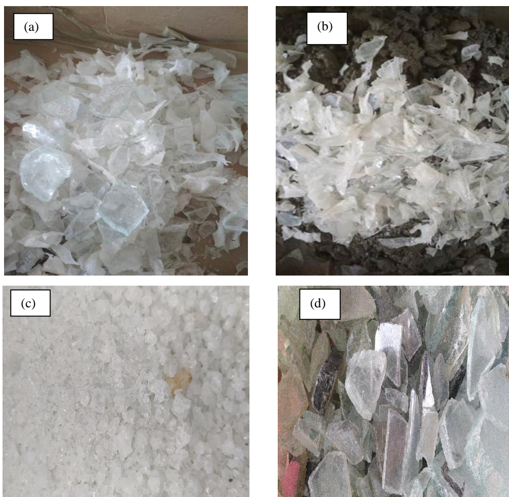
Figure 3. Windows glass (a) and (b) simple glass (SS), (c) and (d) ST 0 – 2 mm, respectively ST 4 - 6 mm
