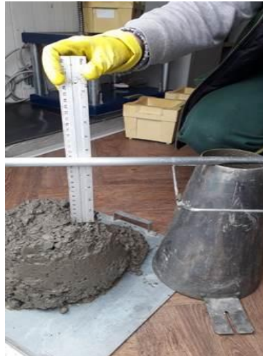
Figure 9. Measurement of settlement during experiments
