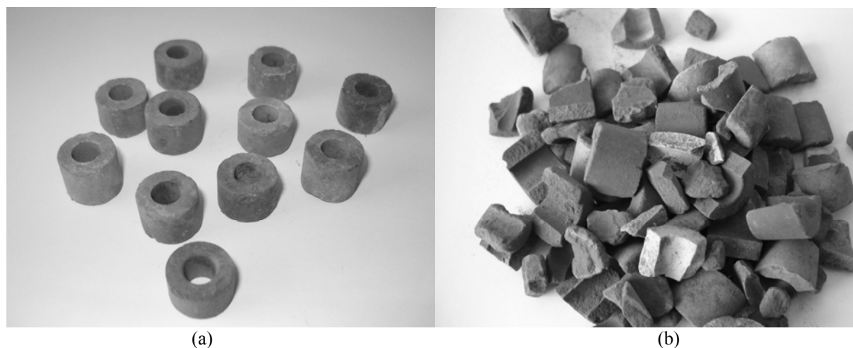
Fig. 1. Natural gas steam reforming catalyst: (a) initial rings; (b) broken and crushed rings after discharge
