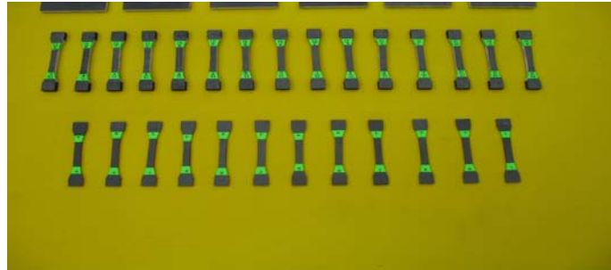
Fig. 4. Specimens used in tensile tests (general view)
