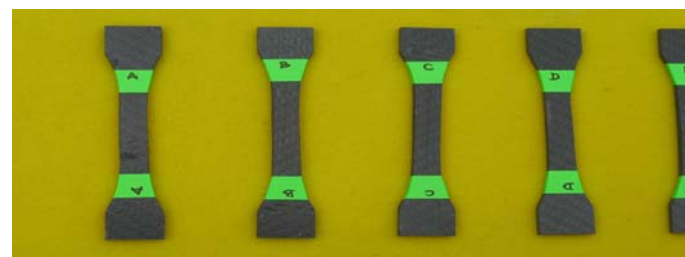
Fig. 6. Specimens type A...L used in tensile tests
