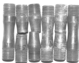
Fig. 2. Test specimens tested to thermomechanical fatigue
