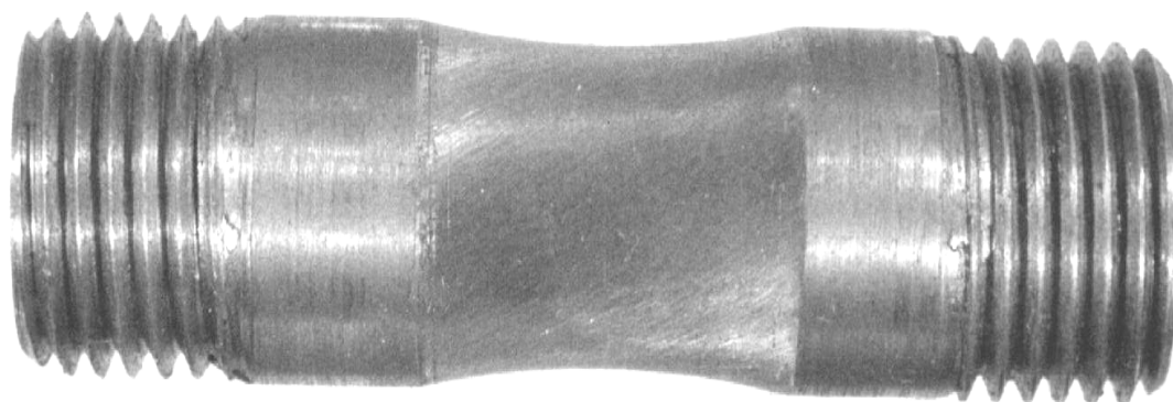
Fig. 2. Test specimen from 16Mo 5.3b
